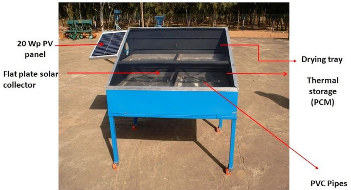
Figure 5: PVT hybrid solar dryer with PCMs [23]
